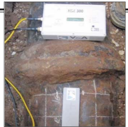
Figure 3. Typical Pulsed Eddy Currents Setup
