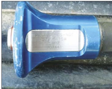
Figure 2. Ultrasonic Thickness Testing Transducer
